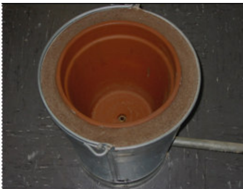
Finished Pellet roaster, minus wire-mesh basket.
