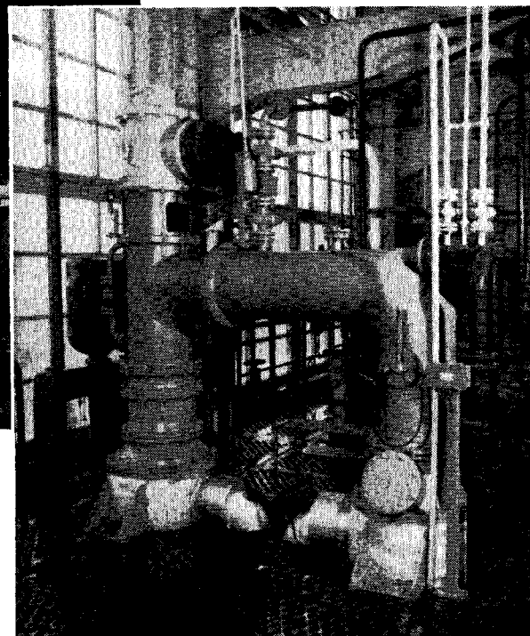
Top of the ethyl acetate reactor. The pump on the upper left hand corner circulates the reaction mixture around the more or less rectangular tube which makes up the vessel. Tops of cooling jackets extend up just above the grating floor
