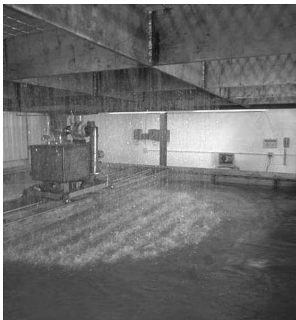
Figure 13 Distributor testing facilities. (Photo courtesy of Koch-Glitsch Inc.)
